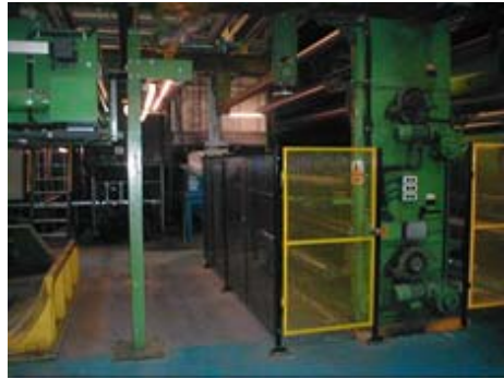
Double Backer Glue Unit 1 Fence with interlocked gates
